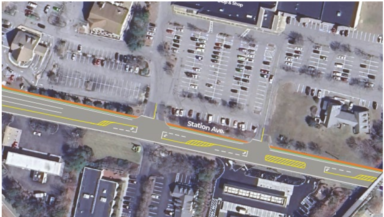
Figure 24: Turn Lane Concept Replacing the Two-Way Left-Turn Lane
