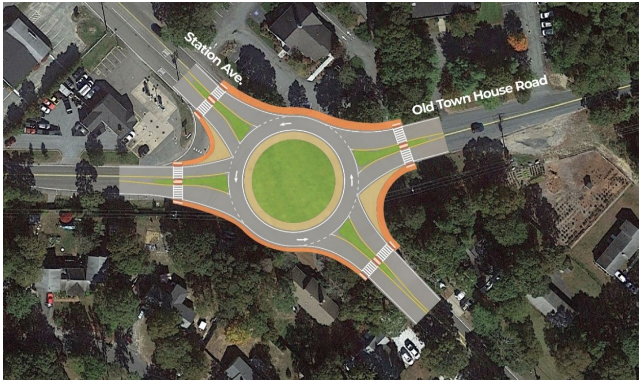
Figure 21: Roundabout Concept at the Station Ave at Old Townhouse Road Intersection- Not Recommended
