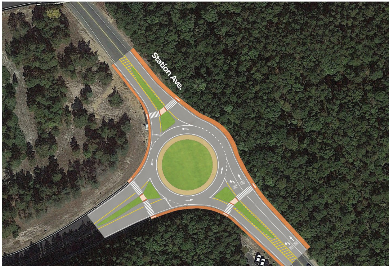
Figure 13: Roundabout Concept at Route 6 Eastbound Ramp at Station Ave
