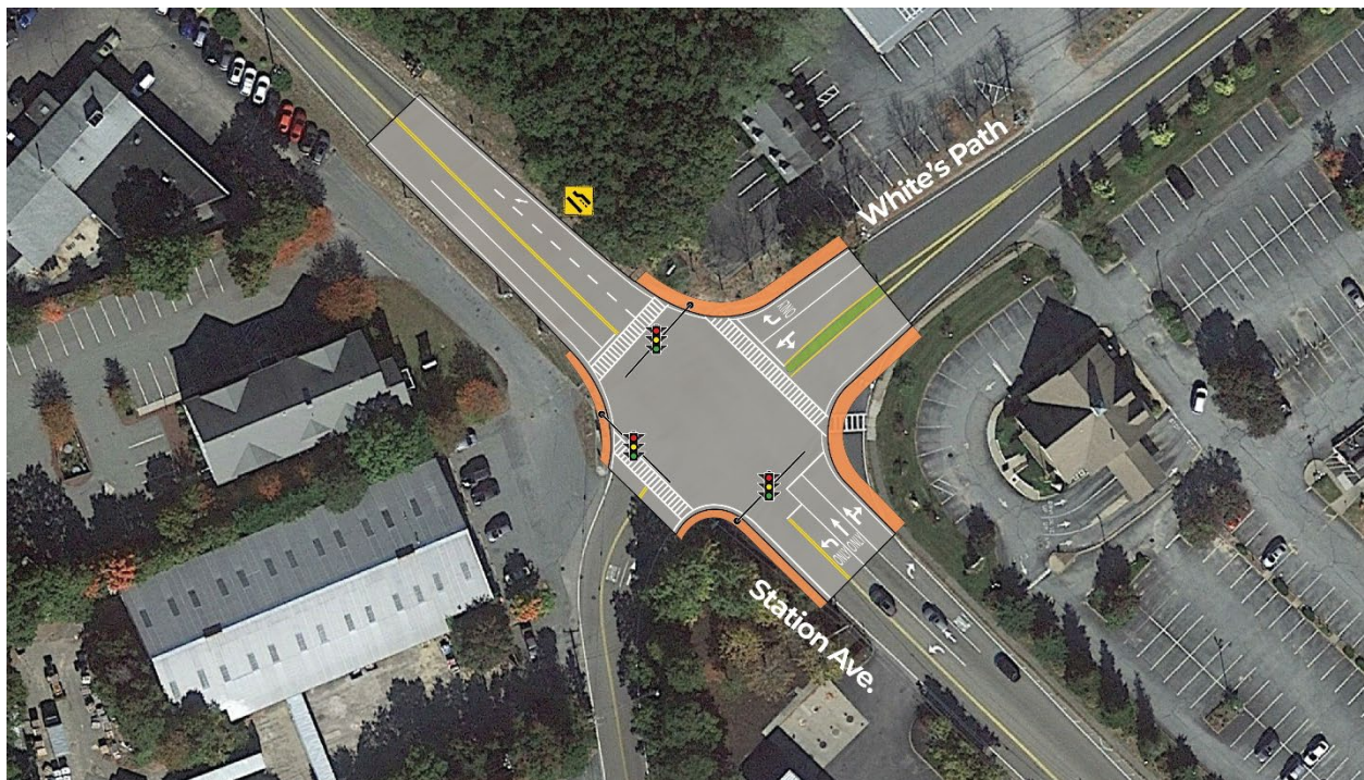
Figure 16: Reconstruction Concept at the Station Ave at White's Path/Workshop Road
