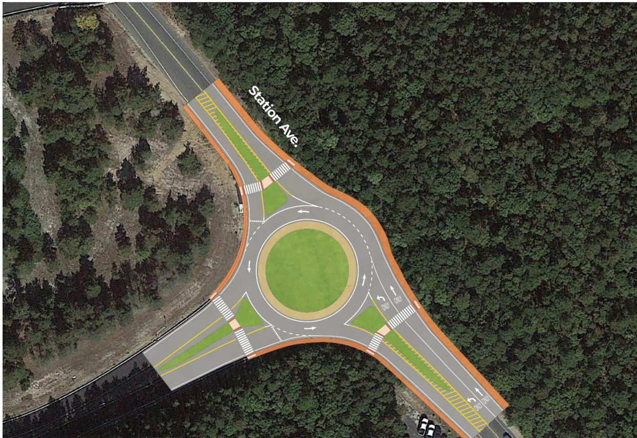
Figure 13: Roundabout Concept at Route 6 Eastbound Ramp at Station Ave
