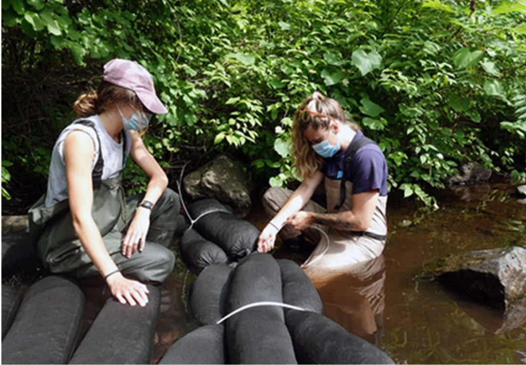
Figure V-5. Biochar socks installed in Lake Hopatcong, NJ. The New Jersey Department of Environmental Protection recently provided a grant to the Lake Hopatcong Commission to test biochar use in an effort to adsorb phosphorus from lake water. Lake Hopatcong is a 14 m deep, ~2,600 acre lake/reservoir with a phosphorus TMDL and a lake management organization, the Lake Hopatcong Commission. Source: https://www.lakehopatcongfoundation.org/news/biochar-installations (accessed 9/5/22).
