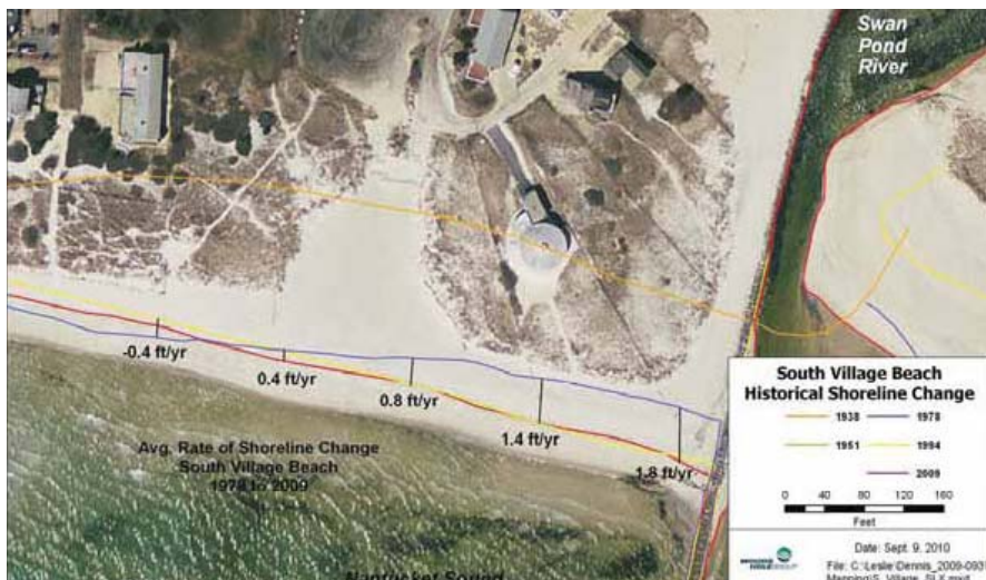
Figure 7: Shoreline change rates east of Lighthouse Inn, at South Village Beach, west of Swan Pond River entrance (WHG 2010).
