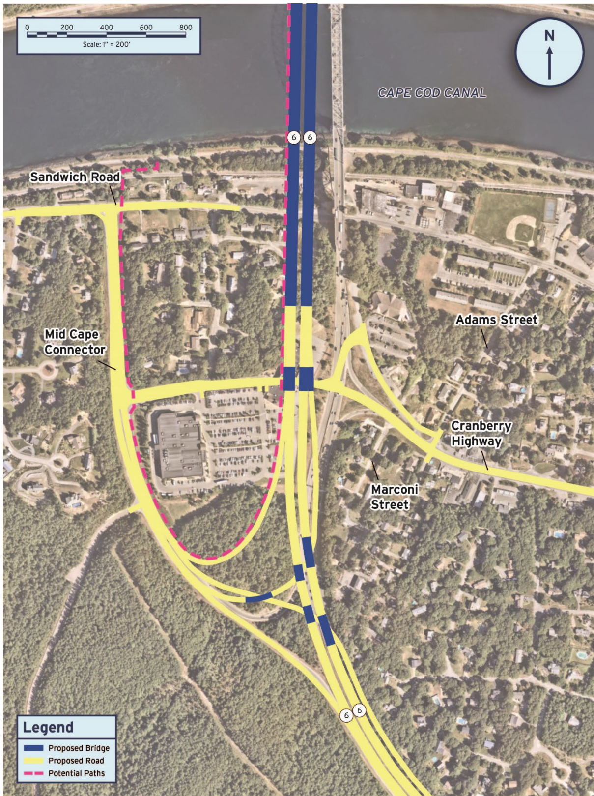
Figure 9-19. Sagamore South Crossing Interchange Approach Option SS-3.1
