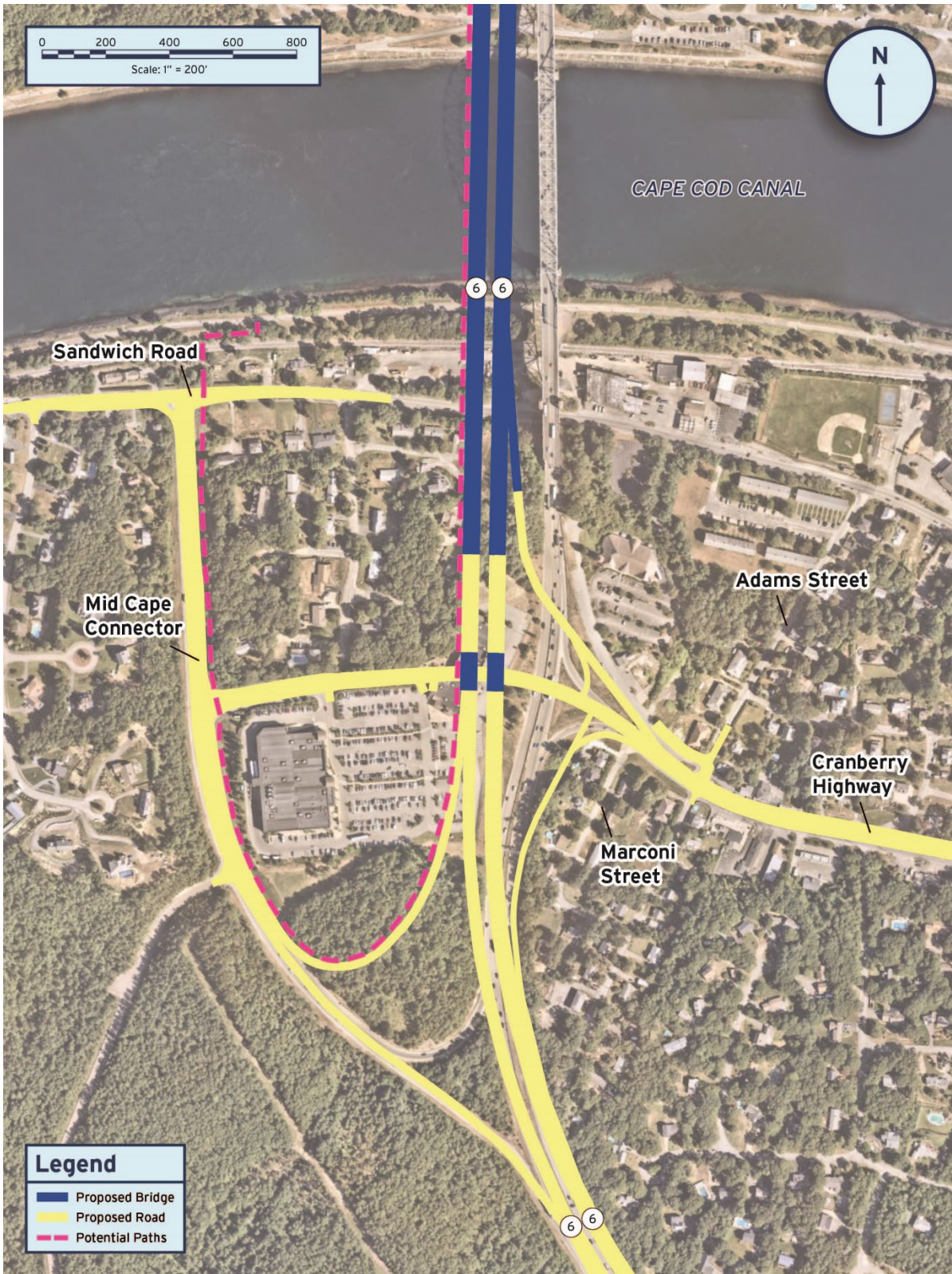
Figure 2-14. Sagamore South Crossing Interchange Approach - Similar to Existing Configuration with Cranberry Highway Extension Alternative
