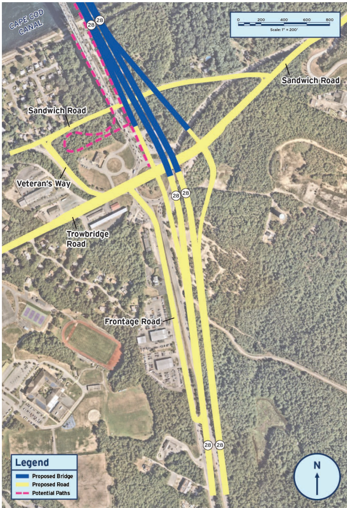
Figure 9-6. Bourne South Crossing Interchange Approach Option BS-2
