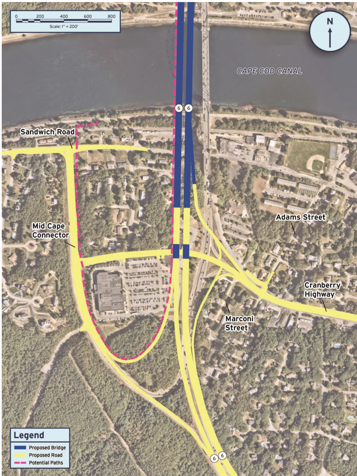
Figure 9-15. Sagamore South Crossing Interchange Approach Option SS-1
