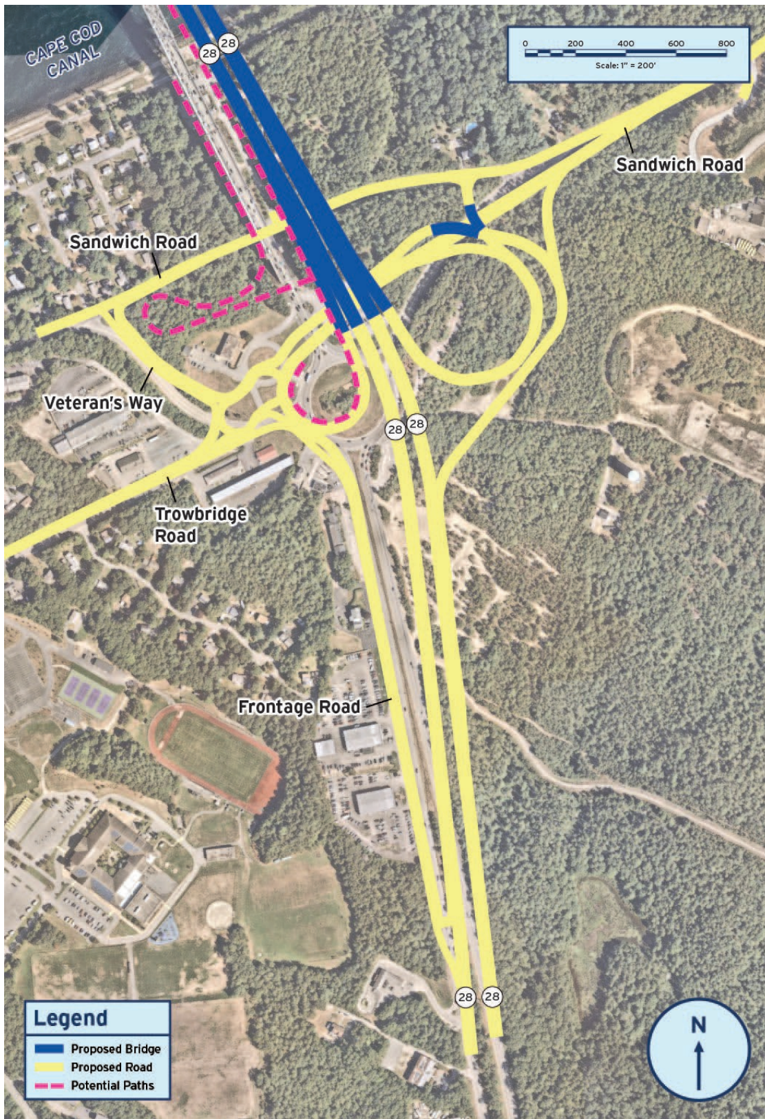
Figure 9-8. Bourne South Crossing Interchange Approach Option BS-6.1
