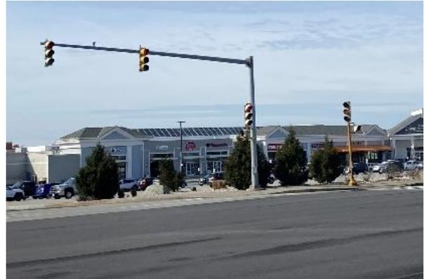
**Image 7: Route 132 at Cape Cod Mall/ Capetown Plaza intersection with outdated signal equipment and no retroreflective back plates on the signals.**
