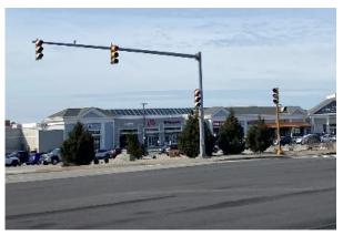
Image 7: Route 132 at Cape Cod Mall/ Capetown Plaza intersection with outdated signal equipment and no retroreflective back plates on the signals.
