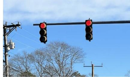
**Image 9: Pitcher’s Way signal heads, faded visors and no backplates.**
