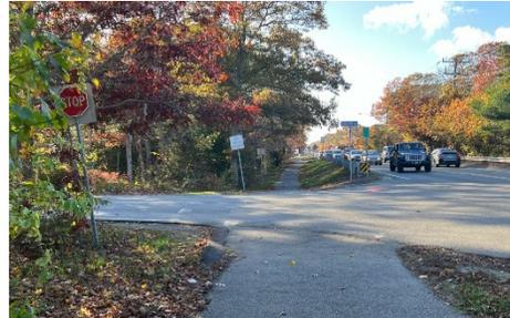
**Image 19: Lack of visibility of the shared use path crossing and guardrail obstructed view.**
