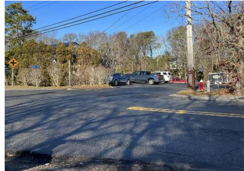
**Image 22: Missing or faded fog line on Route 28, faded stop bar on Lincoln Road Extension and no visible lane markings.**
