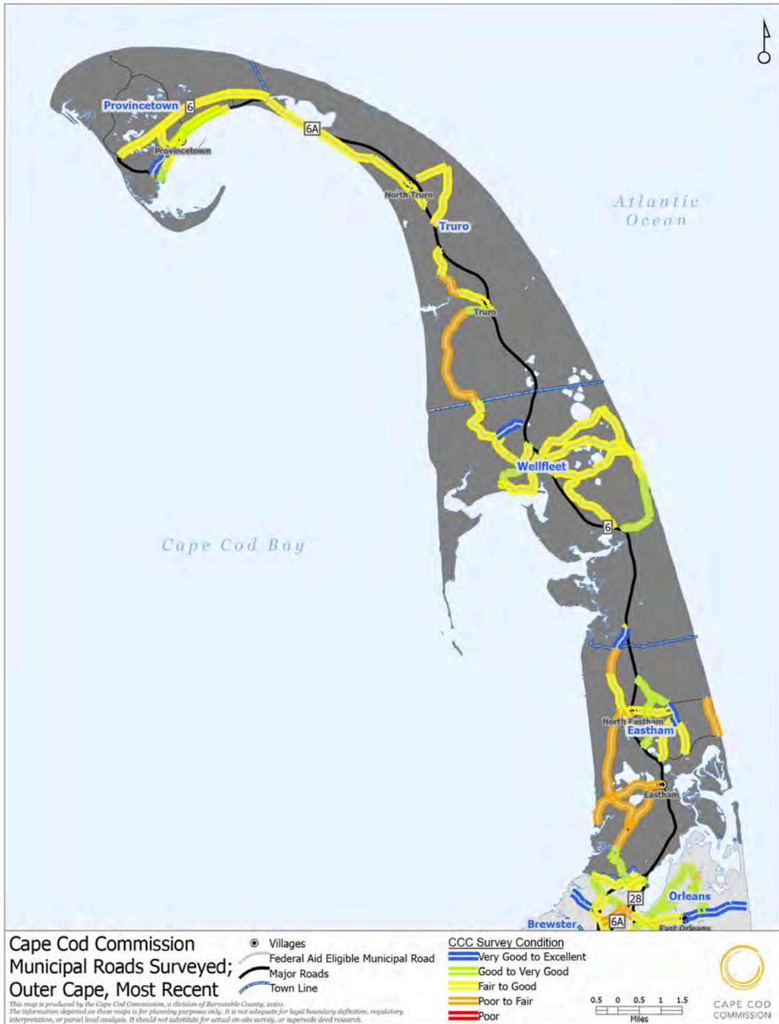
**Figure 6 – Pavement Condition Surveys: Outer Cape**
