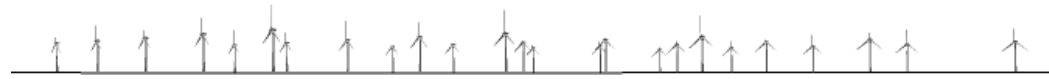
Figure 20: 25 turbines arranged in 5 rows of 5 turbines; when viewed from the side, a more random and less-uniform pattern is seen.
