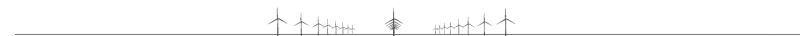
Figure 18: the same 24 turbine array viewed from the side, showing significantly smaller horizon spread.
