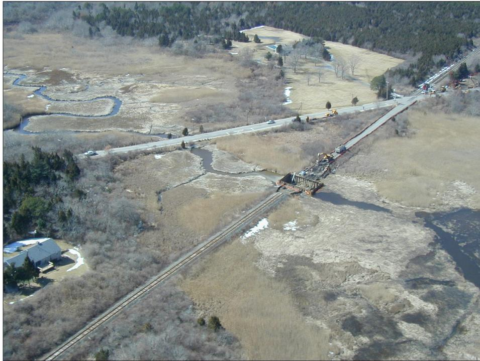
Replacing undersized culverts with larger culverts at the Bridge Creek road and railroad crossings in West Barnstable helped restore tidal flow to 40 acres of coastal wetlands.
