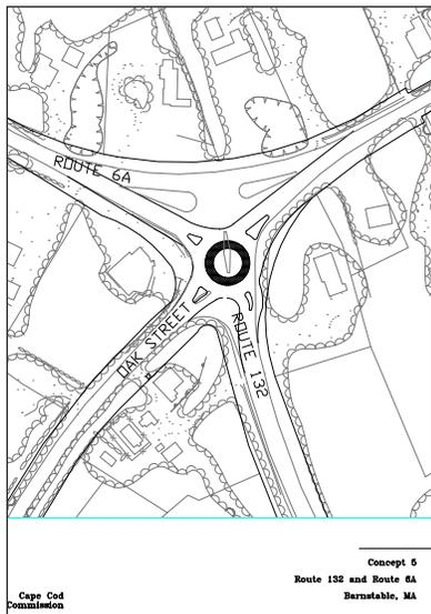
Figure 24 – Diagram of a potential roundabout for the intersection shown in the photo above.
