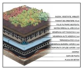
GREEN ROOF COMPONENTS | Photo Credit: Hidroset
