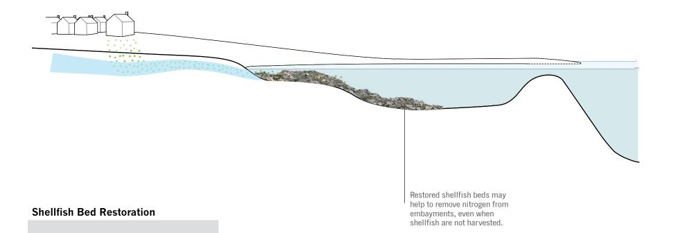
Restored shellfish beds, specifically oysters, can help to remove nitrogen in degraded water bodies. New reefs can be created by depositing old oyster shells and oyster spat into embayments where nitrogen removal is desired.
