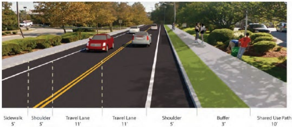
Figure 29. MassDOT Route 28 Corridor Study complete streets recommendations
