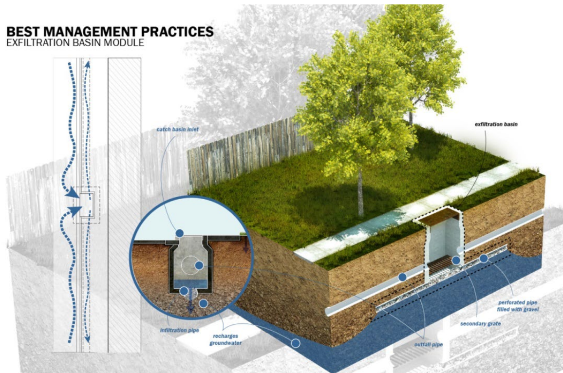
FIGURE 12. Leaching Catch Basin
