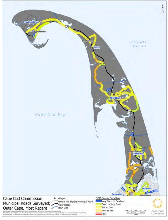
Figure 6 – Pavement Condition Surveys: Outer Cape Source: latest data available from 2018-2020 collected by Cape Cod Commission
