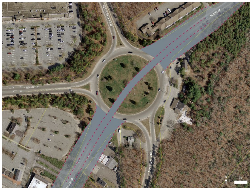
Figure 17. Route 28 Overpass Alternative and Anticipated Impacts
