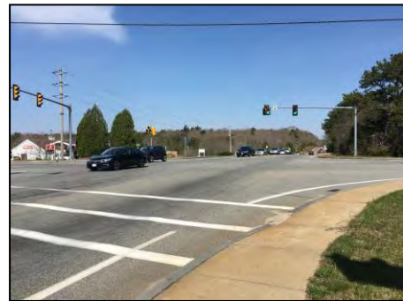
Image 9: Crosswalk across the westbound approach with no ADA ramps or pedestrian signal equipment
