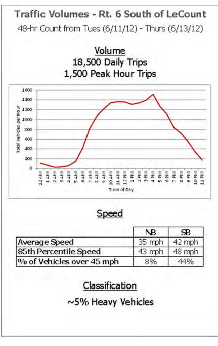
FIGURE 7 - ROUTE 6 AT LECOUNT HOLLOW ROAD: HOURLY TRAFFIC VARIATION, CLASSIFICATION, & SPEED DATA
