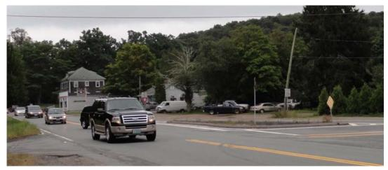
Sandwich Road (Route 6A) at Cranberry Highway, Bourne. Note that second vehicle is pulling over the centerline/cutting the corner to take a left turn. This vehicle may not be visible to Sandwich Road eastbound traffic until it is too late.
