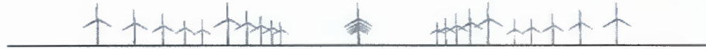
Figure 19: 25 turbines arranged in 5 rows of 5 turbines; when viewed straight on, the grid pattern is easily seen
