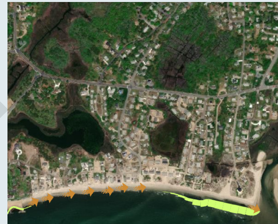
SEDIMENT TRANSPORT DIRECTION AND 40 YEAR EROSION IMPACTS
