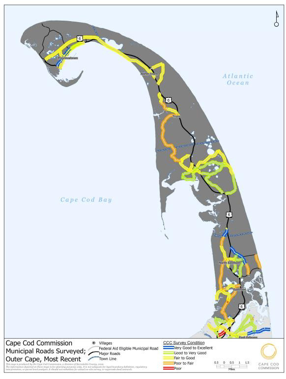
Figure 7 – Pavement Condition Surveys: Outer Cape
