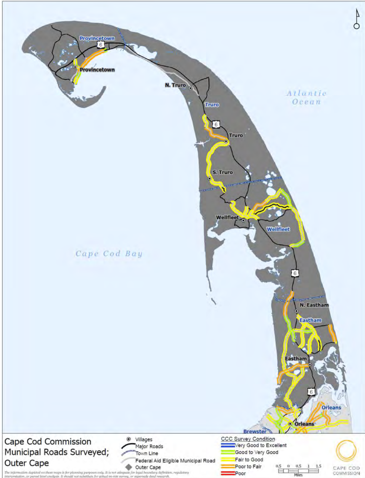
Figure 12 - 2011-2014 CCC Pavement Condition Surveys: Outer Cape
